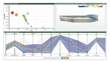
Figure 8: Comparison of contributions from the design constraints for the range of designs highlighted in the upper left plot: size of the deck space small(blue) to large (red).
