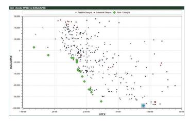
Figure 7: Overview of all investigated designs, with relative CAPEX and OPEX. There are a range of feasible designs (green) that meet the design constraints.
