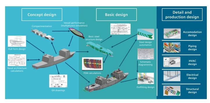
Figure 3: Integrated design environment, with communication both within and between design stages.
