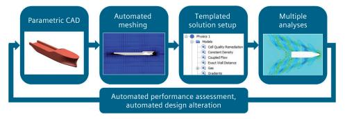
Figure 4: Automated simulation process. Any changes in CAD can be rapidly assessed and the user isn't required to set up models.
